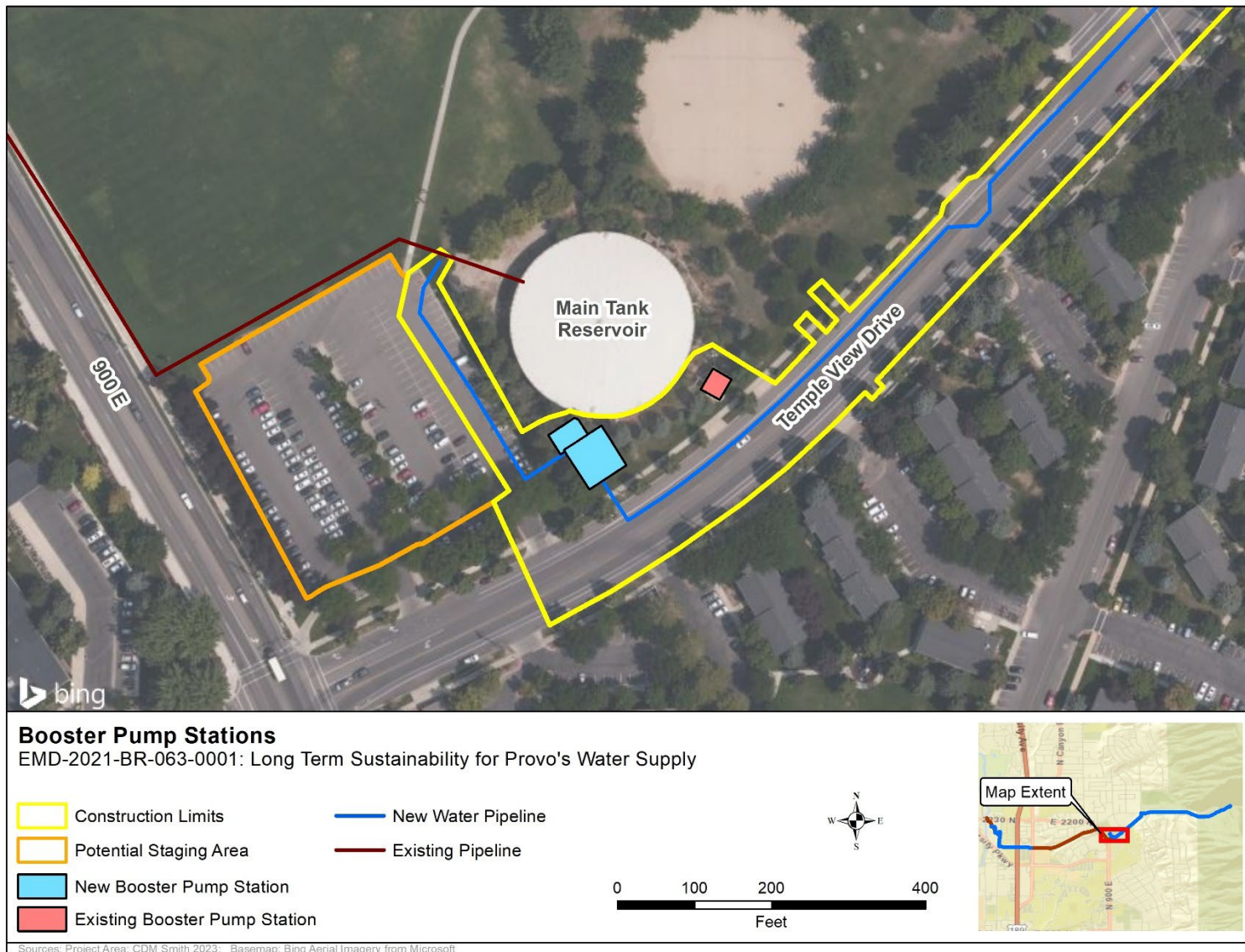
Figure 3-2. Proposed Booster Pump Station
